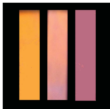
Fig. 5 Fluorescence images of test papers after immersing them in aqueous solutions containing fluoride anions of different concentration. From left to right: 0, 1 and 10 ppm (excited at 365 nm using a UV lamp).
